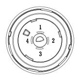
PIN1: 12V PIN2: GND/DIM-PIN3: NC PIN4: DIM+
